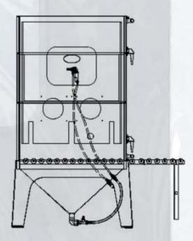
The Venturi system uses less power than pressure systems and is used mainly for engraving at shallow depths, such as for photographs and on glass. The Venturi cabinet joins a pistol to the cabinet hopper forming a closed and continuous circuit for the abrasive.
