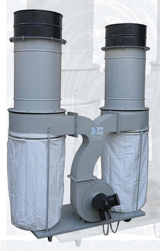
TR suction systems are designed to provide full visibility while engraving in the sandblasting cabinet. They are fitted with motors ranging from 2 to 5.5 hp and a capsule paper filter for a large air flow and a completely hermetic seal to ensure no dust escapes. It features an optional automatic cleaning system which uses blasts of air.
